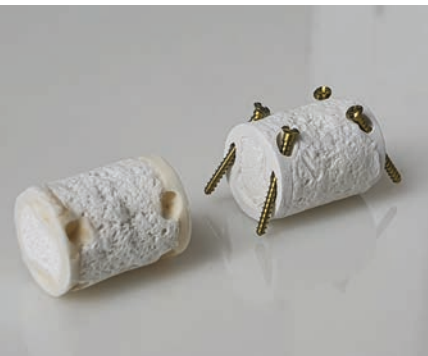
Hybrid bone test samples.
